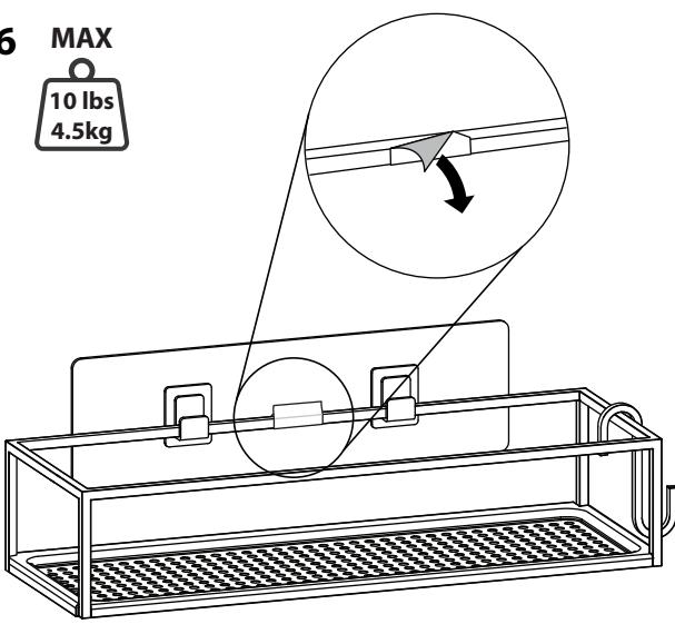
If you need to remove the installed adhesive, you can use a hair dryer to heat the adhesive surface and slowly separate from mounting surface.
